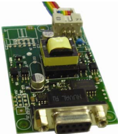
RS-232 communications board
