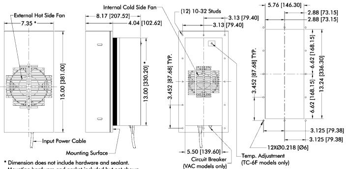
Mounting hardware and gasket included but not shown. Dimensions: Inches [Millimeters]
