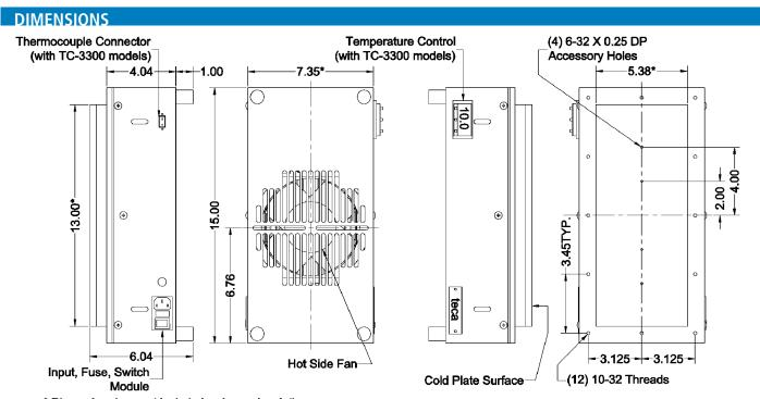
\* Dimension does not include hardware, insulation. **Dimension: Inches**
