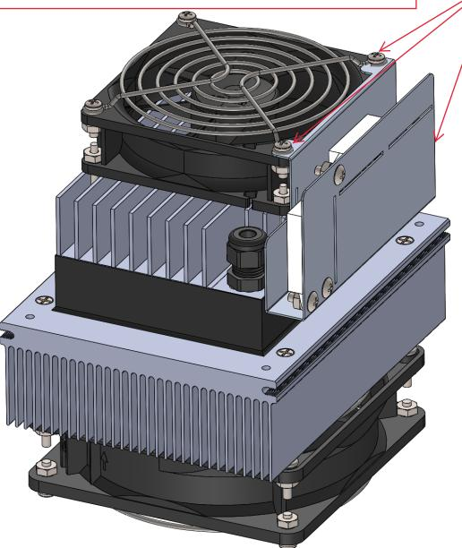
Slide the TC-7F controller bracket under the cold side fan finger guard and retighten the two screws to secure the bracket in place.
