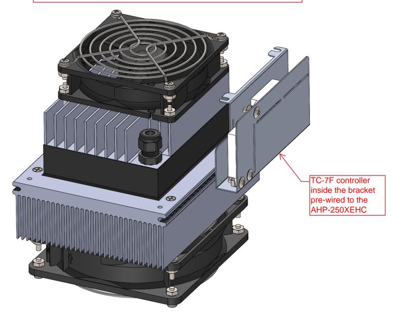
After the installation of the AHP-250XEHC on the enclosure is complete, slide the TC-7F bracket under the cold side fan finger guard and re-tighten the two screws.
