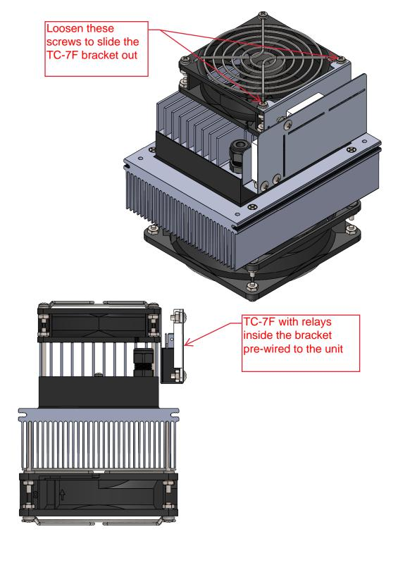
Fit the AHP-250XEHC along with pre-wired TC-7F controller bracket assembly through the mounting cutout on the enclosure. Making sure wires are not pinched between the enclosure and the unit, secure the AHP-250XEHC on the enclosure.
