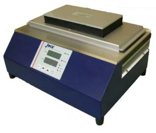
Accessory Plate Clamp: ACP-1200 side clamps can also be used to secure the cascade to the AHP-1200CPV. Side holes in the units accept the clamp mounting screws to secure it in place. Top set screws are used to apply a slight pressure to the cascade securing it in place while avoiding undue compressive forces on the thermoelectrics. The clamps work only for the CCP-22 and CCP-31 Cascades.
