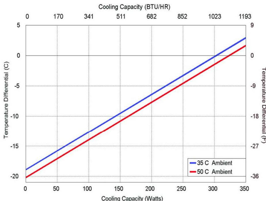
Equation of line:  $y = \Delta T ({}^\circ C)$   $x = \text{Capacity (Watts)}$
