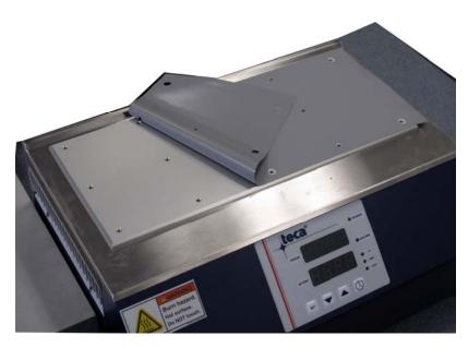
6. Install 3" long 6-32 threaded stud (2 included) 1 per cold plate in the middle hole of each cold plate. This will help assembly of the gradient bar later.
