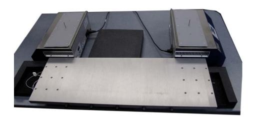
8. Two people, carefully, first line up one stud with mounting hole in the gradient bar then move the 2<sup>nd</sup> CPV cold plate to line up the other stud with it's mounting hole in the gradient bar. Gently lower the gradient bar onto the CPV cold plates. DO NOT DROP THE GRADIENT BAR ON THE CPV COLD PLATES.
