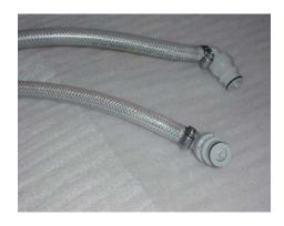
Step 3: Attach both fittings to one hose and then to the TLC-900, forming a closed loop.
